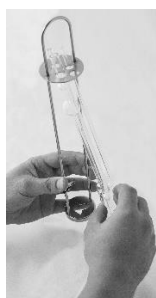
Fig. 4 Inserting or replacing a viscometer with light-barrier sensing
